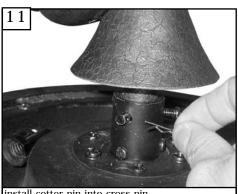
install cotter pin into cross pin.
